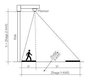
The detection range area y1 can be reduced if the sensor is mounted too close to the pole.
